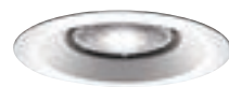
OPEN SHOWER P8072WL-28* White Wet location listed. Metal flange. IC & Non-IC: 50w PAR30* Long Neck *WL trims require use with outdoor rated PAR lamps
