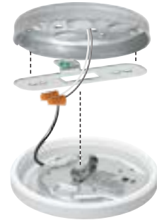
Shown installed into 1/2" ceiling pan J-box
