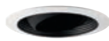
REGRESSED BAFFLED EYEBALL P8079-31 Black Baffle Rotates 358°, tilts 30° max. IC: 65w BR30, 50w PAR30 Non-IC: 75w PAR30, 85w BR30
